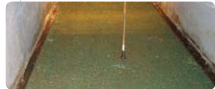
Post-test endurance results concluded that unvegetated GreenArmor 7020 exhibited a critical shear stress of 5.8 lb/ft 2 .
